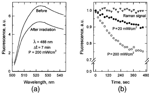
Fig. 3. Bleaching behavior of human skin fluorescence. (a) Fluorescence spectra before and after 7-min illumination at 200-mW/cm<sup>2</sup> intensity. (b) Fluorescence intensities (at 530 nm) and Raman response versus time during irradiation with 488-nm light at 20 and 200-mW/cm<sup>2</sup>. Note that the Raman response stays constant, whereas the fluorescence bleaches with time.
