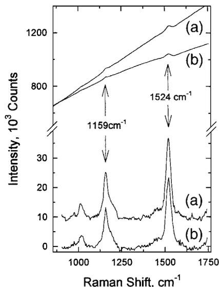
Fig. 2. Typical Raman spectra for (a) human forearm skin and (b) oral cavity tissue, measured *in vivo*. Top traces, spectra obtained before subtraction of native fluorescence background; bottom traces, after subtraction.
